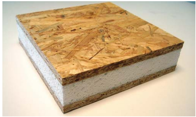
(Fig.1) A typical wood structural insulated panel (SIP) is made of two oriented strand board (OSB) skins sandwiching an insulating foam core, most commonly expanded polystyrene (EPS) (shown).
