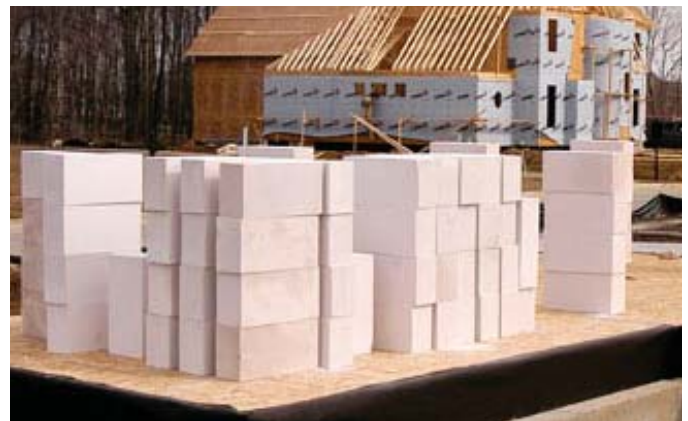
(FIG.C) AUTOCLAVED AERATED CONCRETE (AAC) has a uniform texture that can be left exposed for interior finishes. Exterior sides of walls should be protected from weather.
